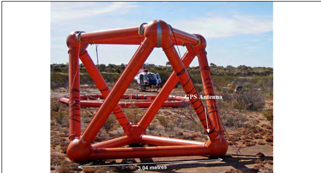
Figure 3. ZTEM and AirMt base station sensor.
