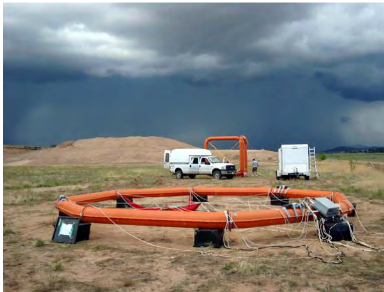
Figure 1: ZTEM Hz Receiver Coil (foreground) and Hx-Hy Reference Coils (background)
