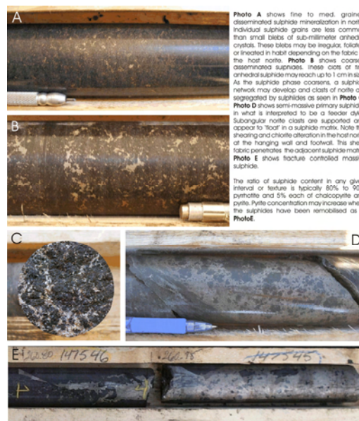
Figure 4: Slide showing texture of sulphides in Axis Lake diamond drill core (after Vivian and Lo, 2007).
