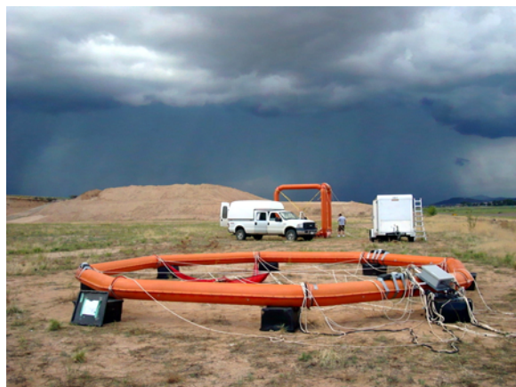
Figure 2: ZTEM AFMAG Hz Receiver Coil (foreground) and Hx-Hy Reference Coils (background)
